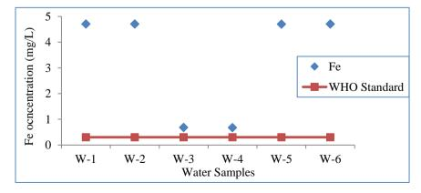
Figure 2 Fe concentration in water samples
